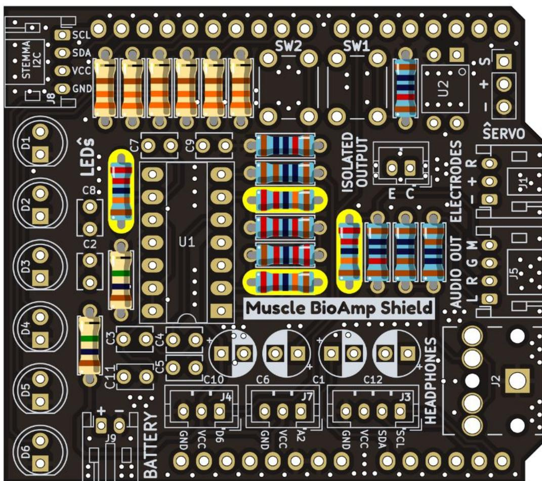
Fig. 14: Step 7 - 220K Resistors
