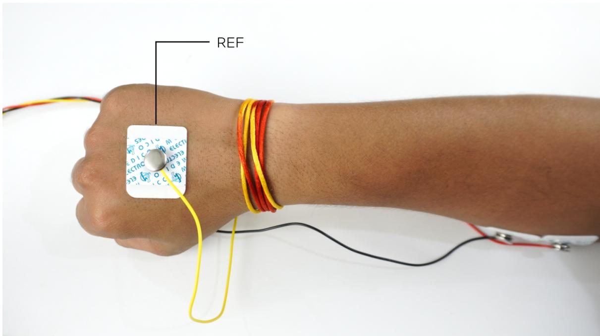
Fig. 32: Electrode placement for REF cable
