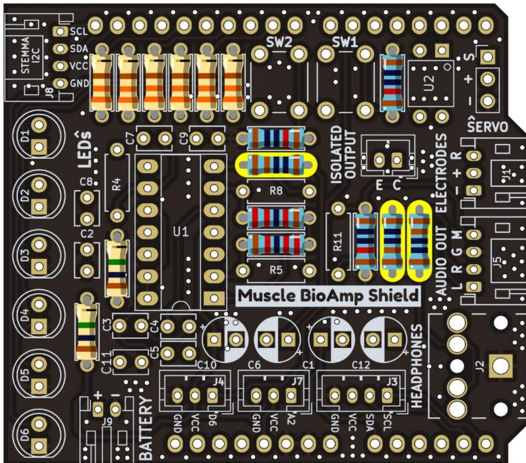
Fig. 13: Step 6 - 1K Resistors
