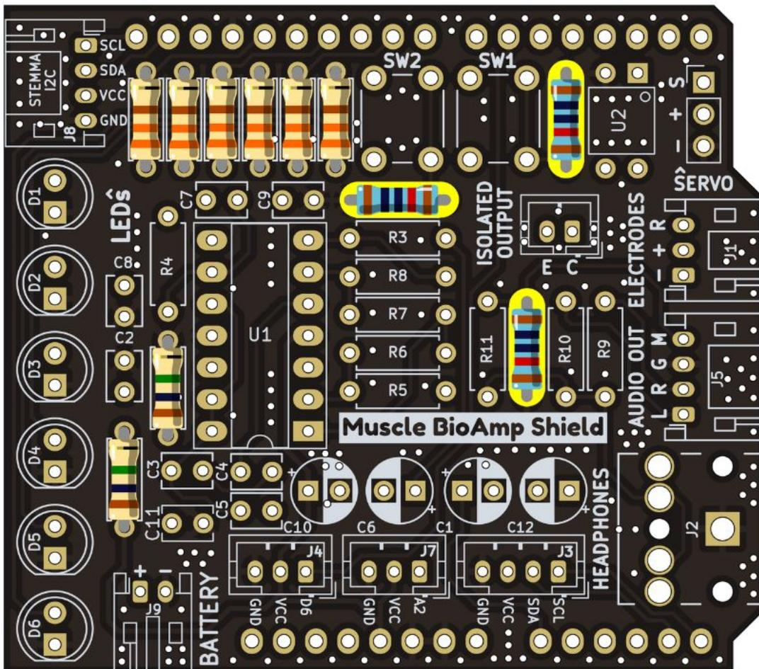
Fig. 11: Step 4 - 10K Resistors
