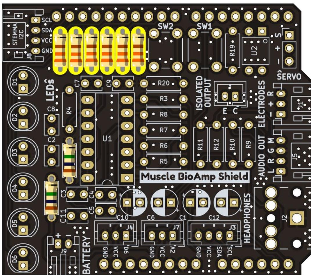
Fig. 10: Step 3 - 330R Resistors
