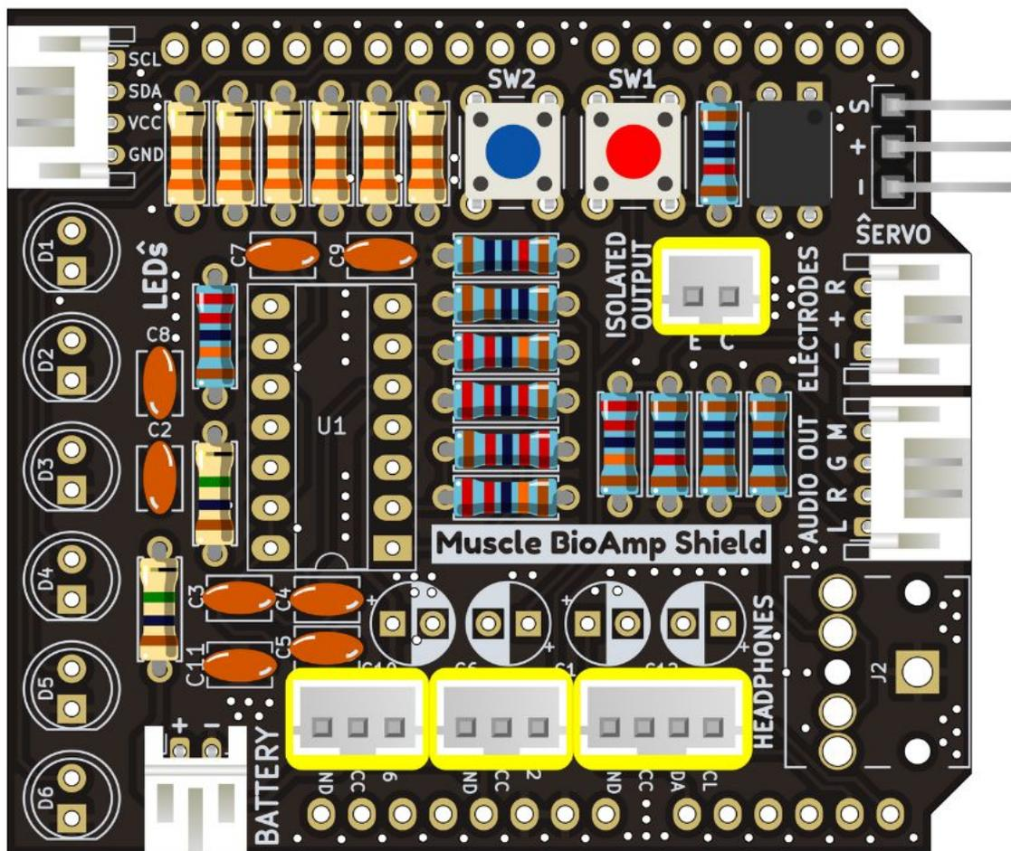
Fig. 22: Step 15 - JST PH Straight Connectors
