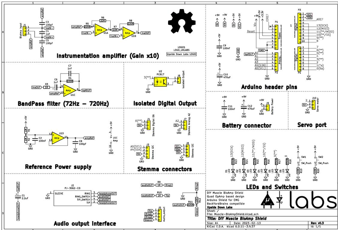
Fig. 5: Schematic Diagram
