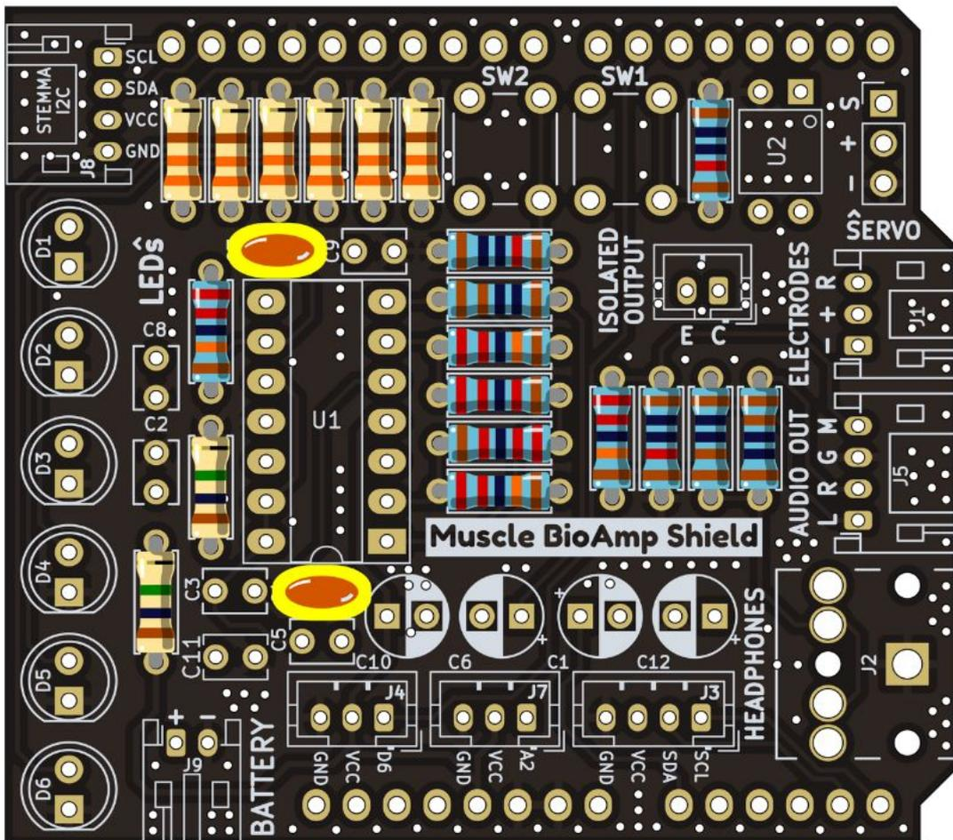
Fig. 15: Step 8 - 1nF Capacitors
