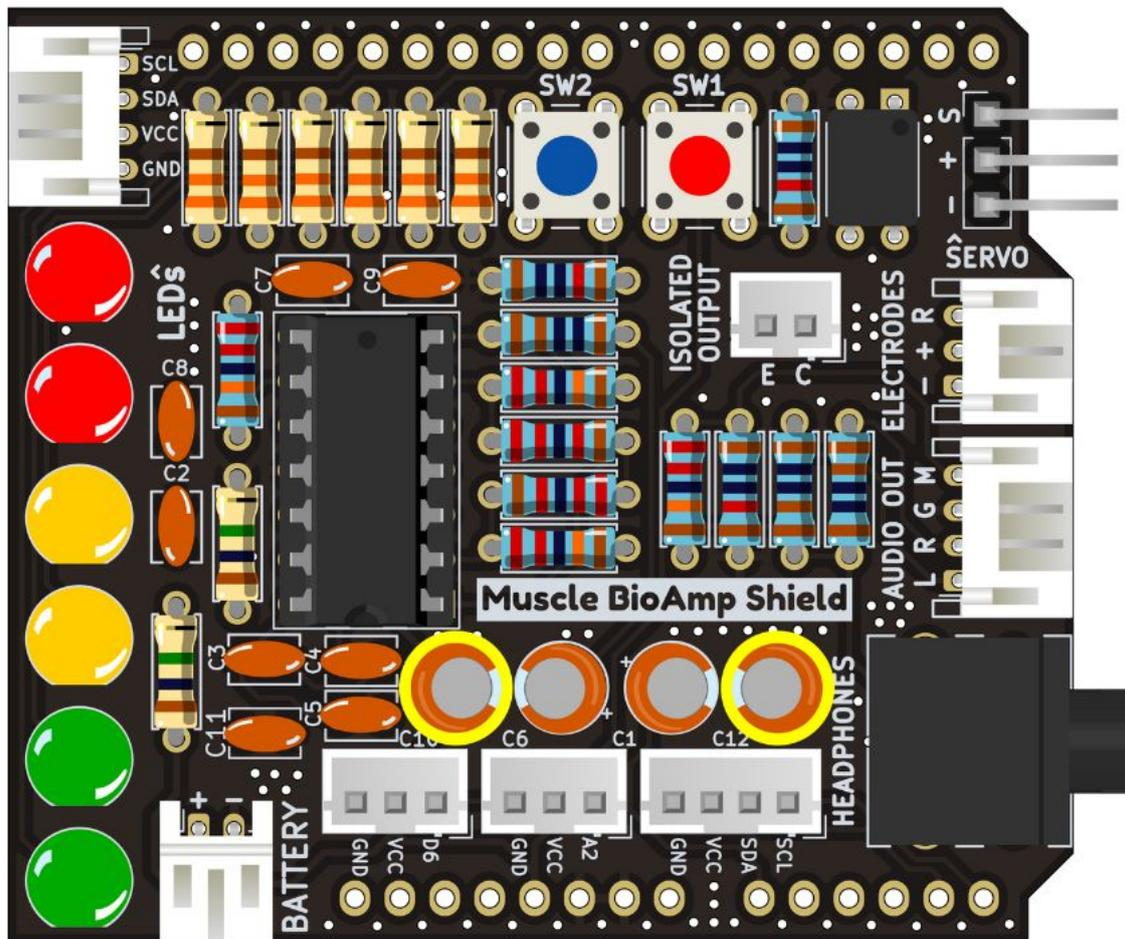
Fig. 29: Step 22 - 470uF Capacitor
