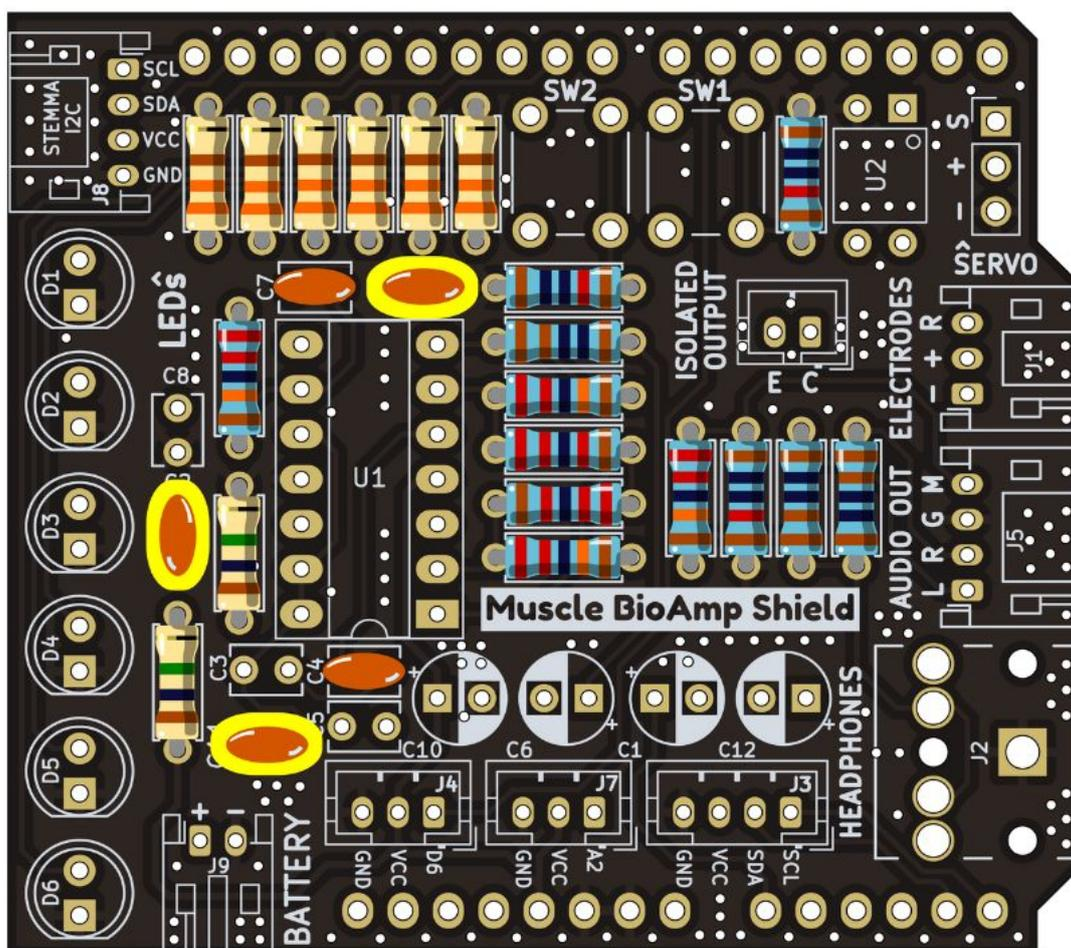
Fig. 16: Step 9 - 100nF Capacitors
