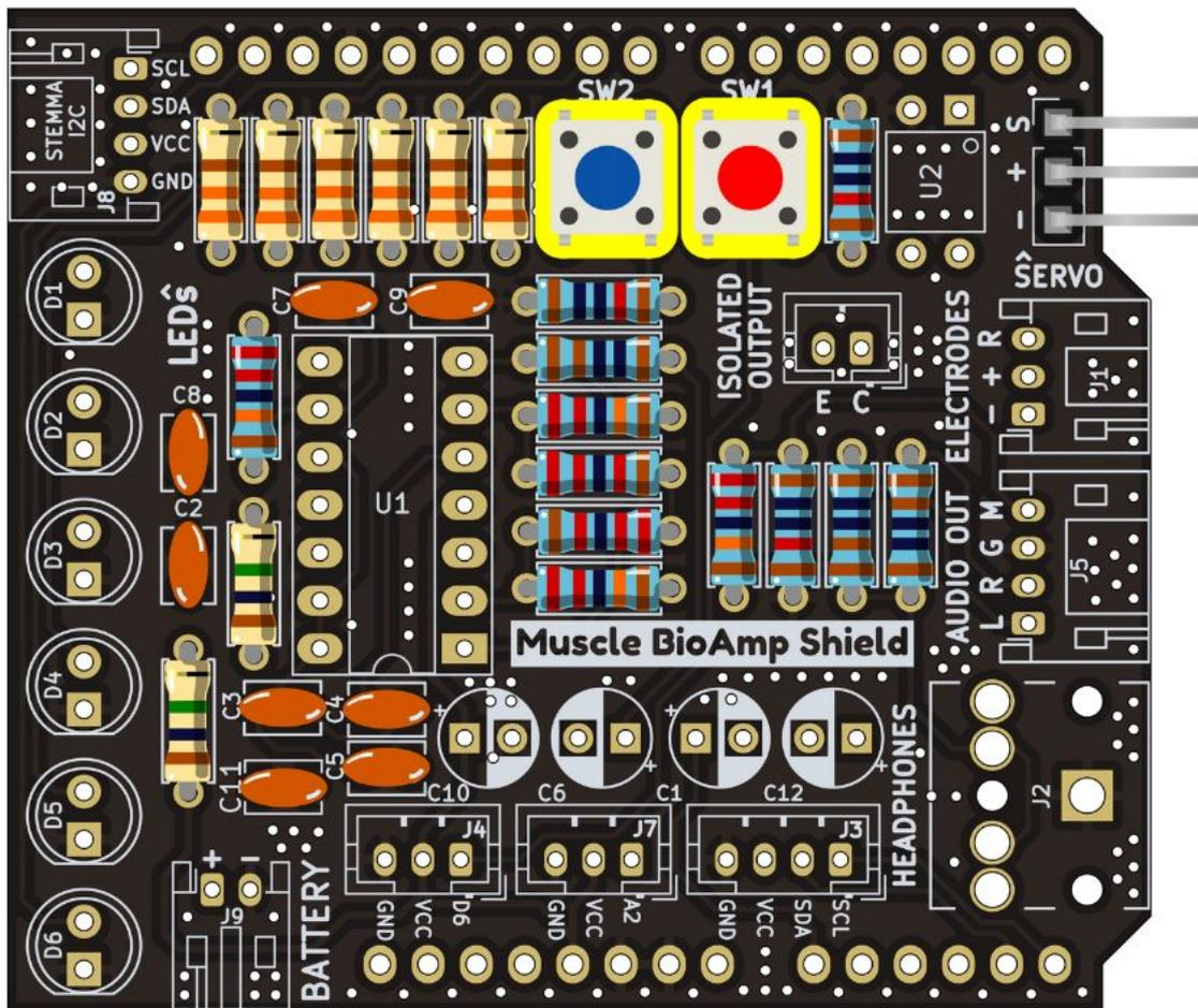
Fig. 19: Step 12 - 5x5mm Buttons
