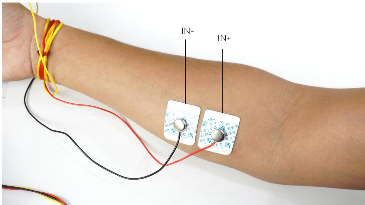
Fig. 33: Electrode placement for IN+, IN- cables
