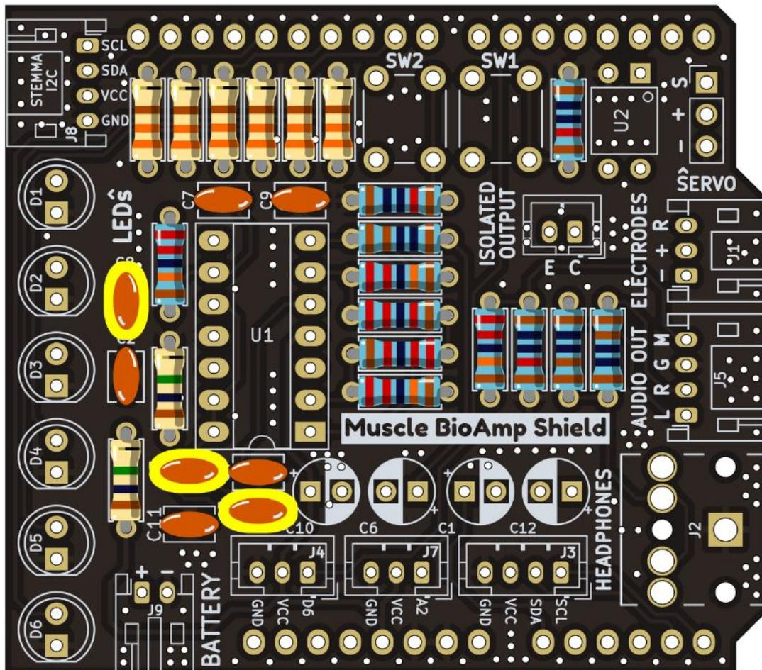
Fig. 17: Step 10 - 100pF Capacitors
