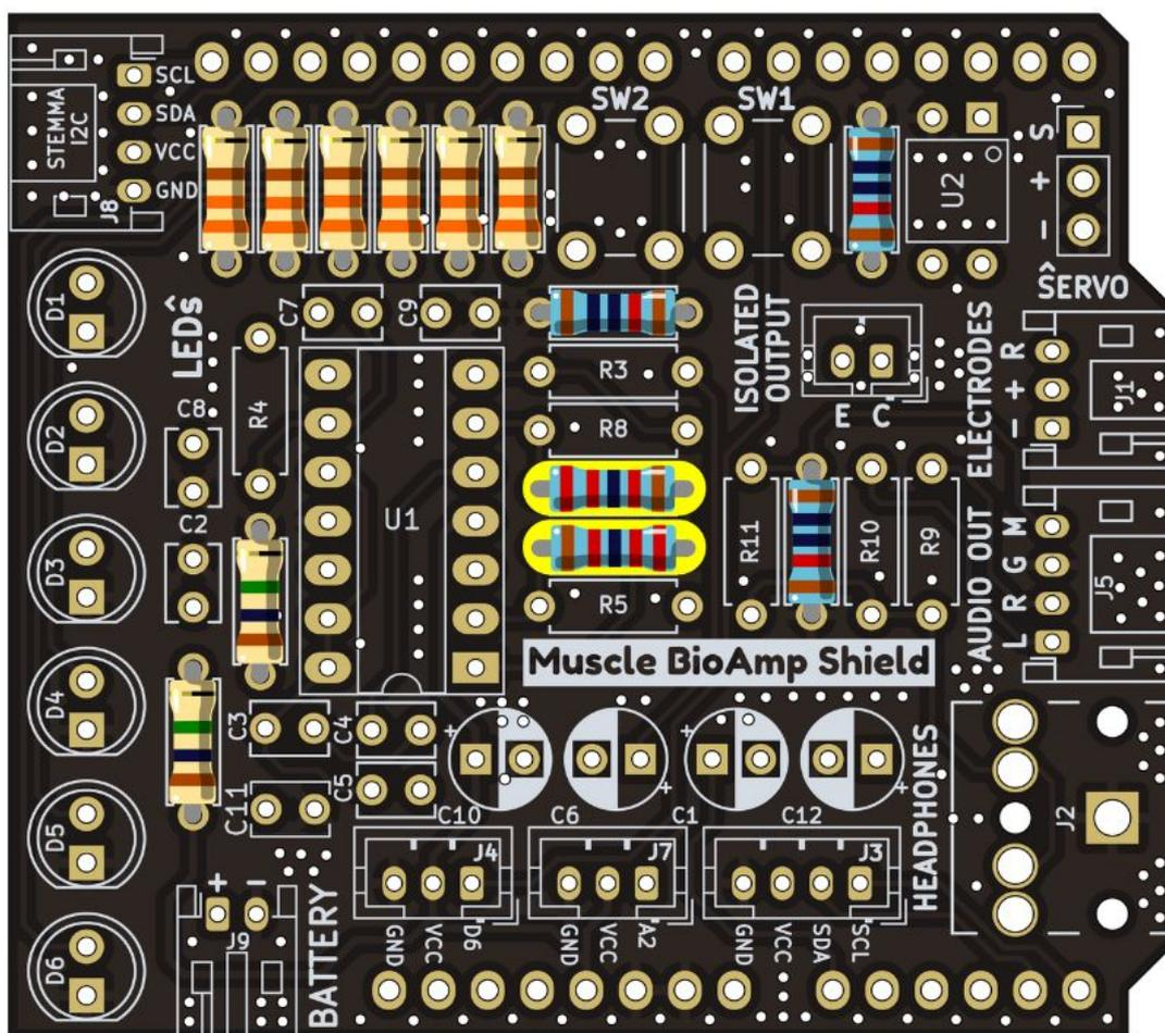
Fig. 12: Step 5 - 22K Resistors
