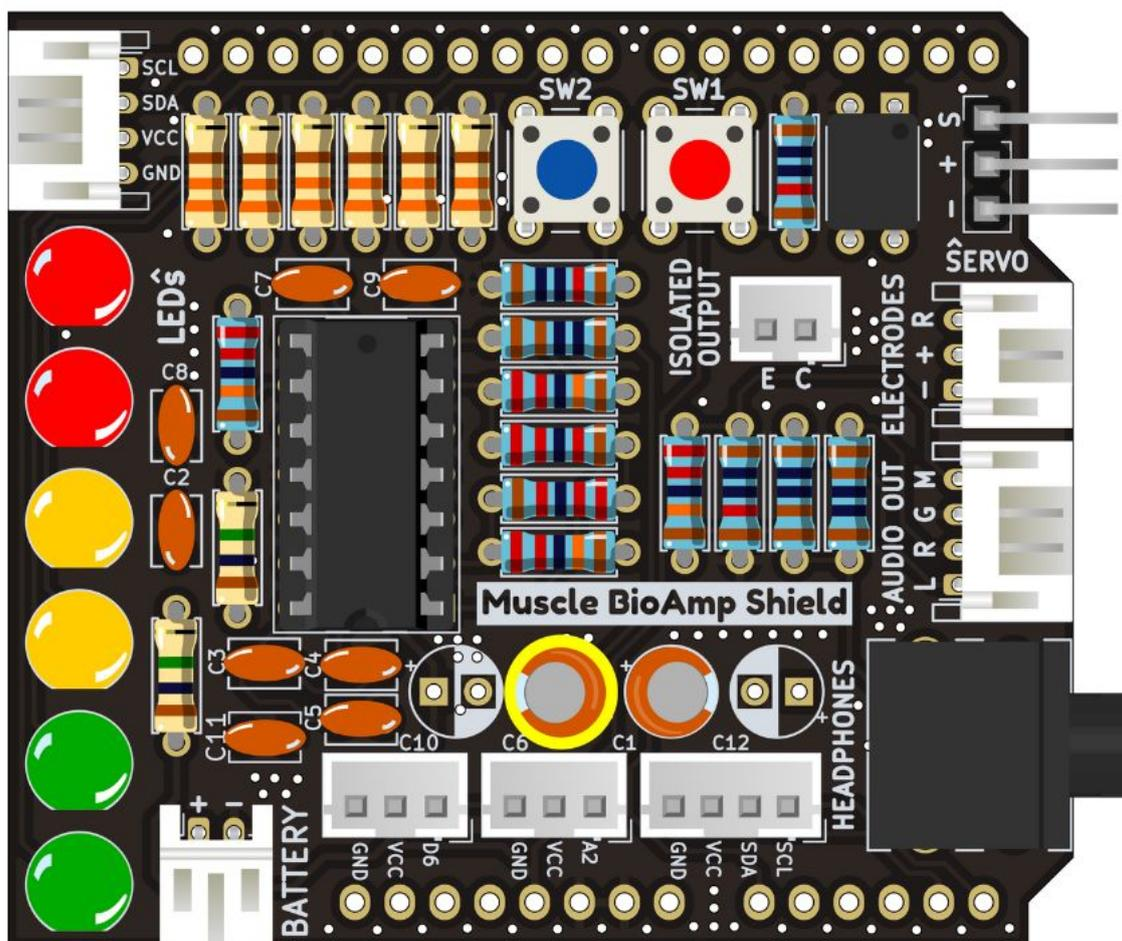
Fig. 28: Step 21 - 1uF Capacitor
