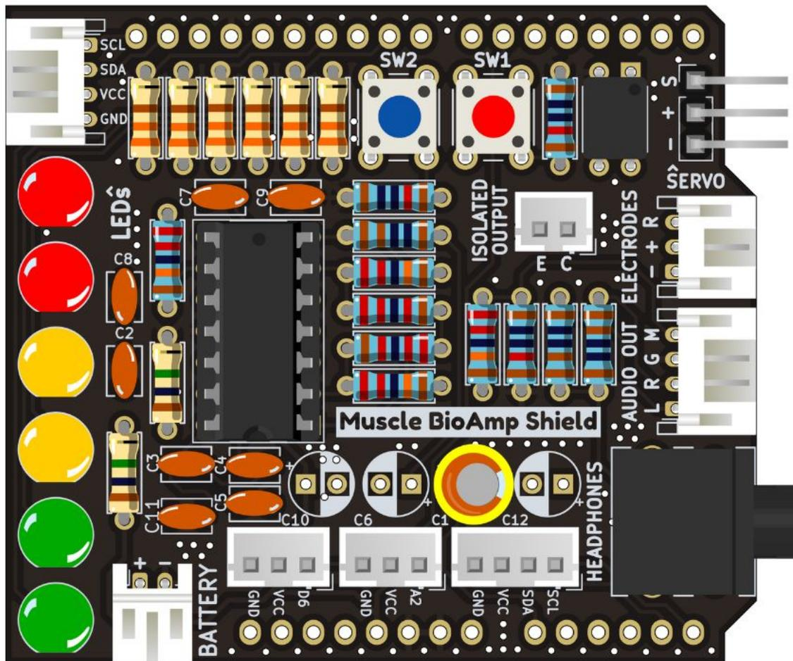
Fig. 27: Step 20 - 2.2uF Capacitor
