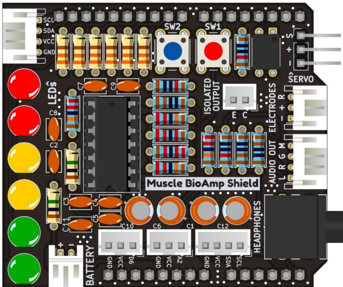
Fig. 31: Step 24 - Assembled Shield
