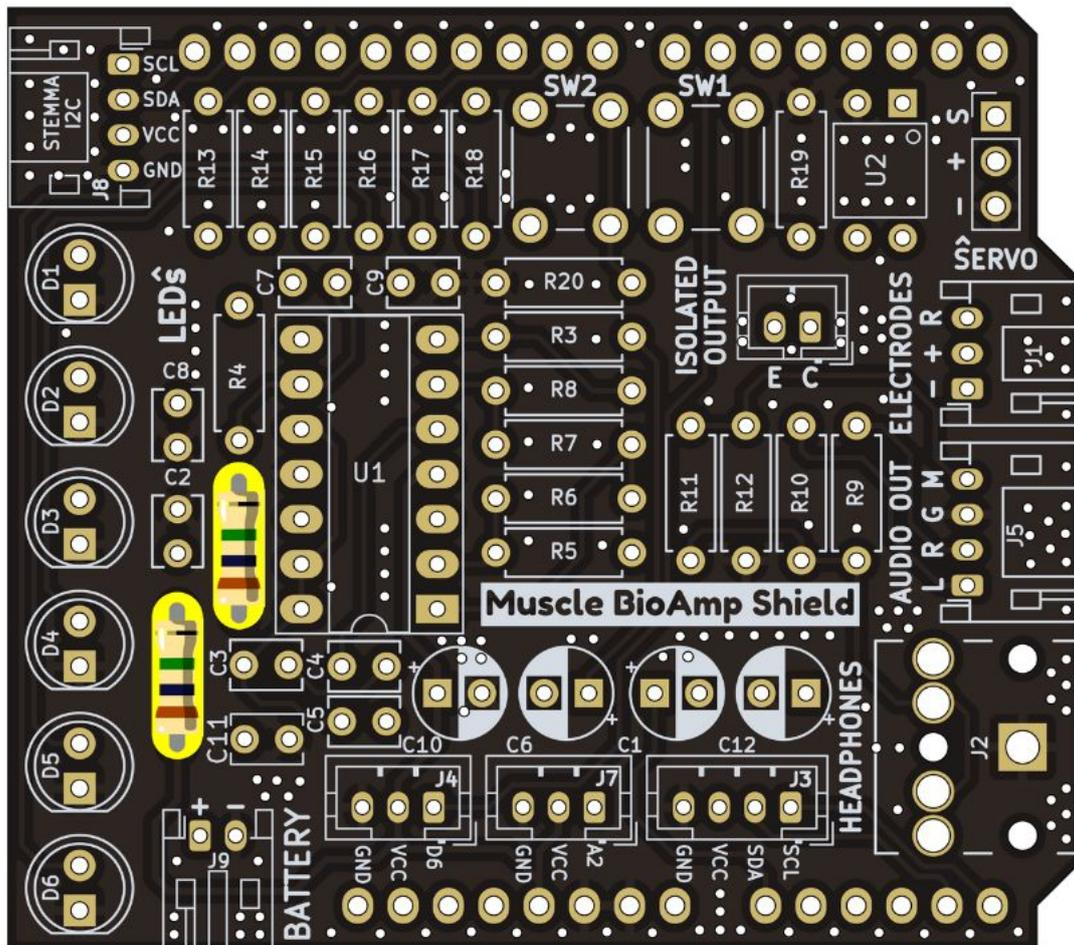
Fig. 9: Step 2 - 1M Resistors
