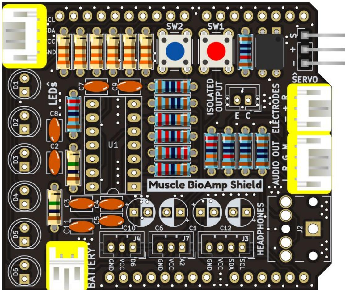
Fig. 21: Step 14 - JST PH Angled Connectors
